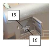
Remove the included 4GB card by pressing onto its end. It will pop out of its slot (15) as shown on the image. Gently remove the card and replace it with the new one by pressing it forward until it is securely locked in the slot. Close the compartment door and lock it by sliding the latch to the left.
