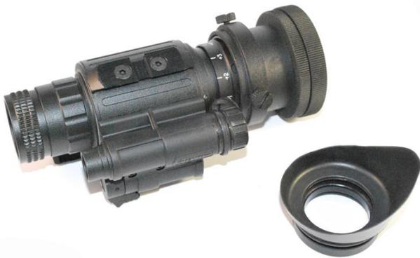
To use the photo adapter first remove the rubber eyecup from the night vision monocular (not the entire ocular, just the rubber eyecup, as seen on the picture on the left) by pulling the eyecup from the ring of the ocular assembly.
