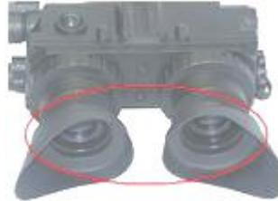
between the eyepieces. If the image appears as if parts of the display are covered, then you need to either pull apart the eyepieces or push them in together until the image appears as one complete display.
